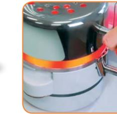
After preheating for approx. 1 minute, swivel the heater over the material.
