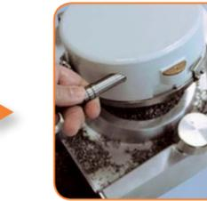
Once the heating time has elapsed, flip the pressure chamber or plate carrier over the model and seal.
