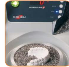
Place model on the platform or embed it into pellets and fix material with the locking ring.
