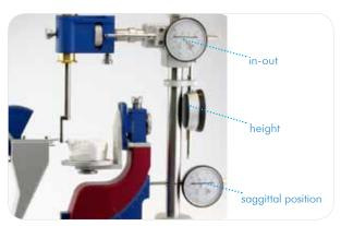
Bond the bracket with composite and take note of the height and the in-out
