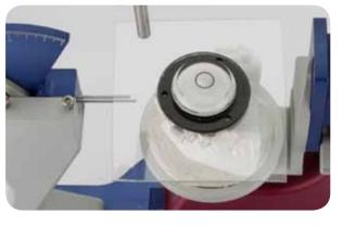
Occlusal Plane leveling with transparent plate and level with bubble in center
