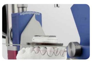
With horizontal occlusal plane, adapt the positioner to the dental axis
