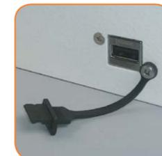
Free accessible USB port with protection cap for simple software updating.
